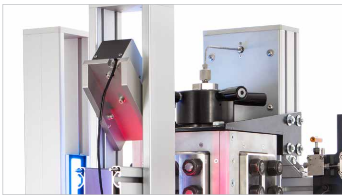
Camera recording foam structure
