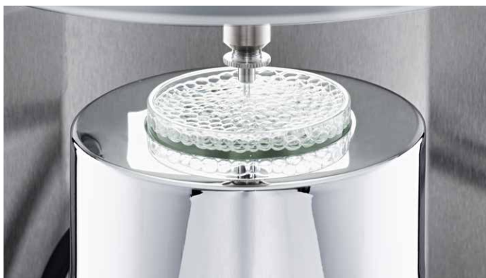
Sample stage with integrated temperature control
