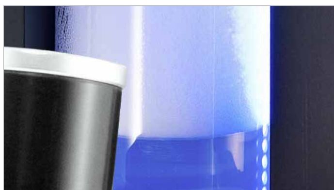
Detection of liquid-foam-boundary
