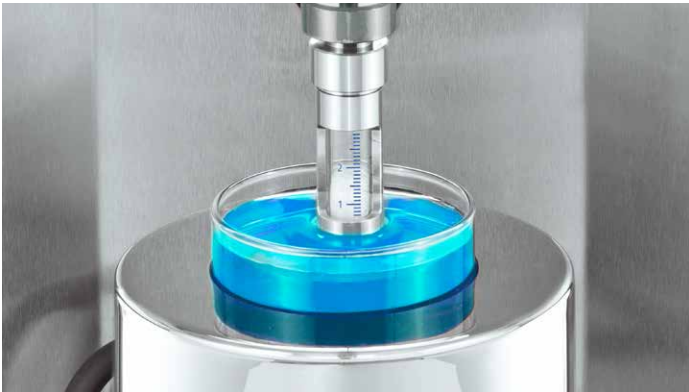
Washburn method for powder contact angle measurement
