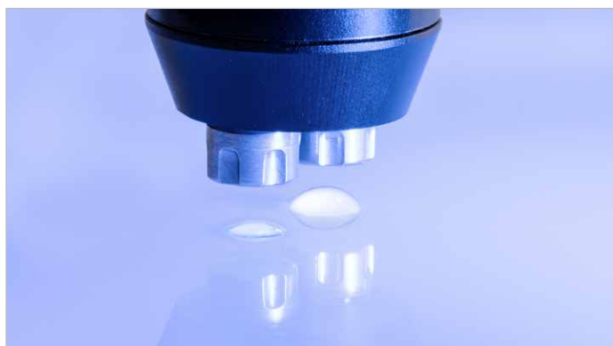
SFE measurement with two drops using the Liquid Needle
